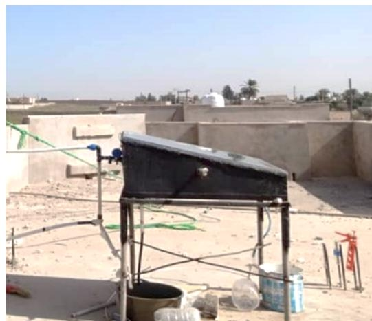
**Figure 2.2 On-site Image of the Vacuum-assisted Solar Still**
