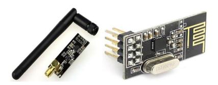
Figure I: Transceiver nRF24L01
