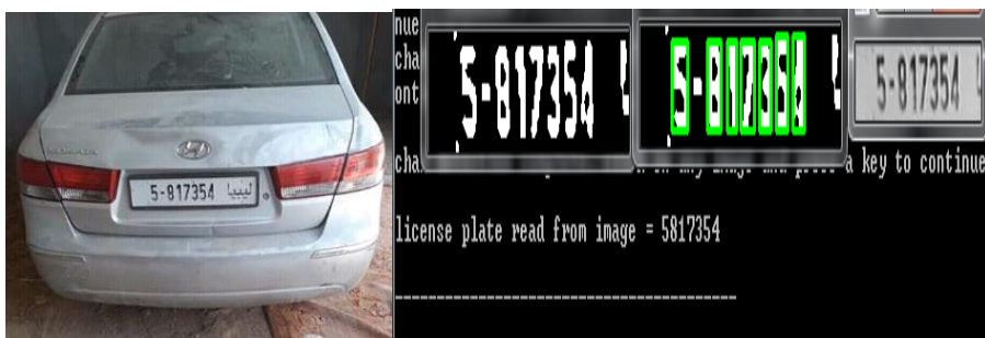
Figure 11(a) Image with Dust or Some Oils Covering the Lower Half of the Plate, (b) Results
