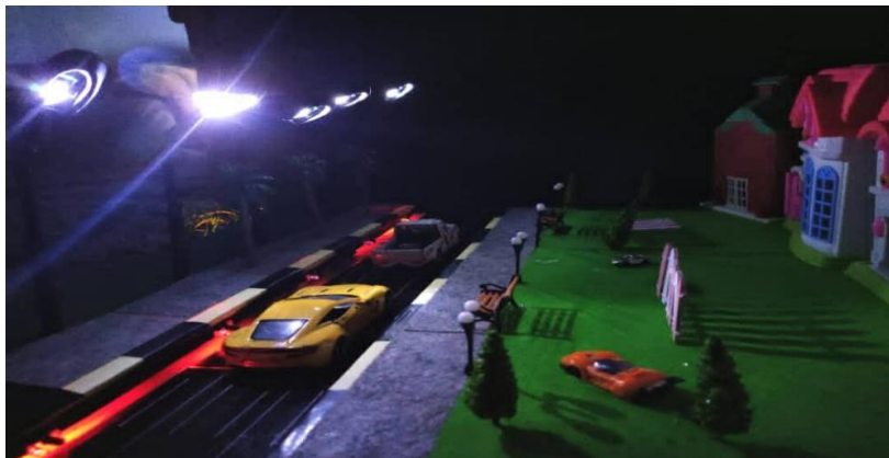
Figure 10: Smart Street When There's no Movement Outside Shows Dimming Lights
